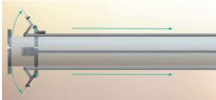
Fig. 12 Airbrake Deployment Mechanism
